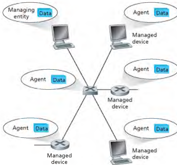
Figure 9.2 ♦ Principal components of a network management architecture
