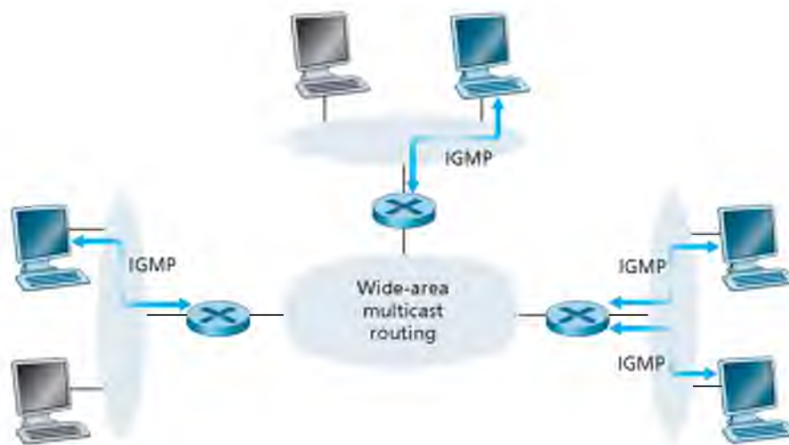
Figure 4.48 ♦ The two components of network-layer multicast in the Internet: IGMP and multicast routing protocols
